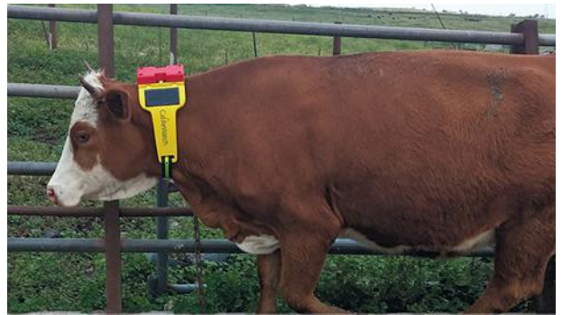
2. The CattleWatch system even broadcasts alerts if predatory animals or poachers are detected. (Courtesy of CattleWatch)
