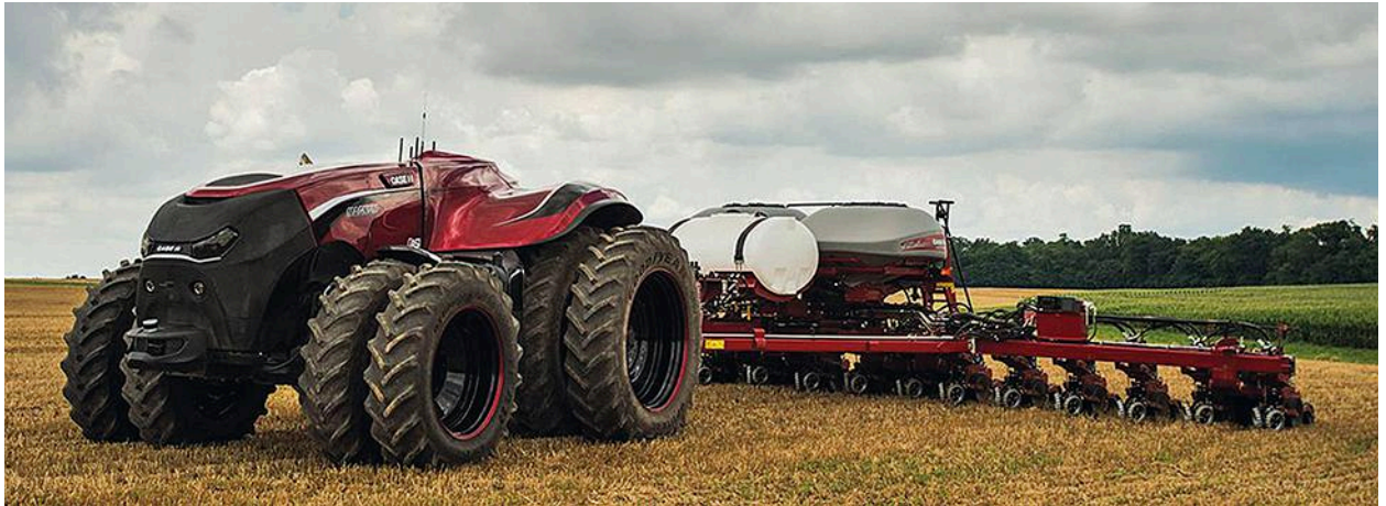
Case IH's concept tractor uses onboard video cameras and LiDAR (light imaging, detection, and ranging) sensors to identify obstacles in its path.
